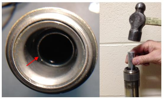
REMOVE TUBE INNER RUBBER SEAL.
