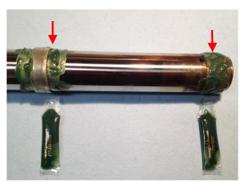
GREASE BOTH BEARING SURFACES WITH THE GREASE PROVIDED OR SOME OTHER HIGH TEMP GREASE. THIS WILL PROVIDE THE LUBRICATION SINCE OIL WILL NOT BE ADDED TO THE SHOCK. ALSO GREASE THE TUBE SEAL.
