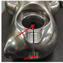
THE RIGHT TUBE WILL NEED TO BE MODIFIED TO MATCH THE LEFT FORK. A THRU HOLE AND COUNTER BORE MUST BE ADDED PER THE DRAWING
