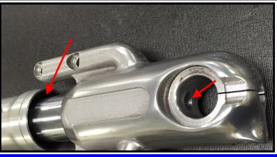
INSERT THE INNER TUBE INTO THE OUTER TUBE. INSTALL THE SLEEVE BEARING AND SEAL AND SECURE THE BOTTOM BOLT IN THE AXLE AREA WITH AN IMPACT GUN. SECURE THE TOP BOLT INTO THE OUTER TUBE.
