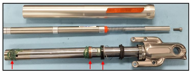
GREASE BOTH THE BEARING ON THE INNER TUBE AND THE UPPER PART OF THE INNER TUBE.
