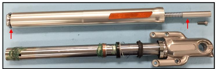
INSERT THE CARTRIDGE INTO THE OUTER TUBE AND PARTIALLY THREAD IN THE TOP BOLT.
