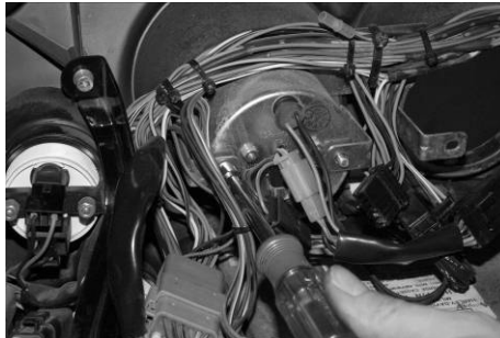
Remove nuts/screws and clamp to remove factory gauges
