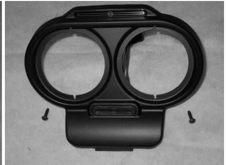
Gauges and gaskets removed
