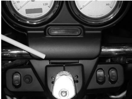
Tab (switch cover removed)
