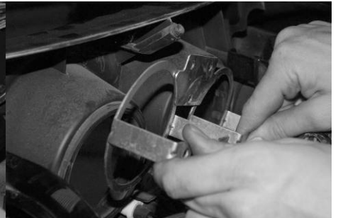
Remove nuts/screws and clamp to remove factory gauges
