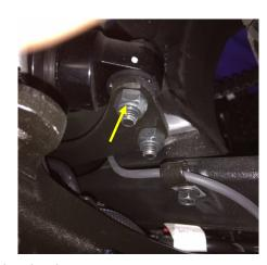
1. Support the bike with a jack stand under the engine, lift to remove the load on the shock. 2. Remove the shock.
