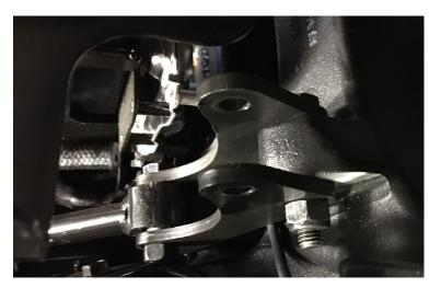
3. Replace the links, note that the long tab secures an electrical connector 4. Re-install the stock shock or the air ride shock.
