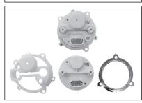
6.The Fuel and Volt bezels and mounting cups will be reused. There are 3 tabs on the bezels that need to be carefully pushed back through the mounting cup to separate the bezel from the mounting cup and to release the factory gauge.
