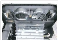
5. Ensure the Speed and Tach bezels remain in the fairing.
