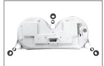
8.Remove the bushings and nuts from the original Speedometer and Tachometer.
