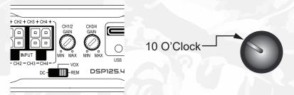
On ALL Low Pass channels - Pre Set GAINs to about the 12 to 1:00 O'Clock position. Typically bass needs more GAIN and more energy to keep up with the mids and highs. This "Pre" set is just that. A Pre set. Its just to get you on your way. ALL settings can me "massaged" and changed at any time
