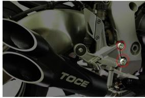
12.) Be sure there is at least a ¼ inch gap between the canister assembly and the swing arm.
