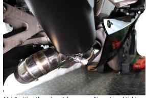
11.) Position the exhaust for proper fitment, and tighten the two bolts on the foot peg bracket
