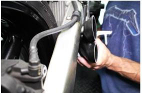
13.) Position the canister assembly in place and install and tighten the canister assembly nut and bolt.
