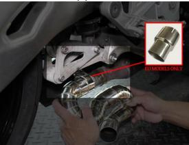
10.) Loosely attach the Toce Canister to the midpipe with the clamp over the inlet pipe.
