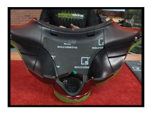
1. Start with piece 1 and place it in the center of the fairing kit above the headlight.
