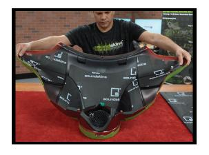
3. Piece 3 and 4 will go on the upper left and right sides of the fairing. Place piece 3 on the top and piece 4 on the bottom.
