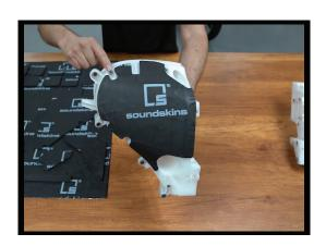
1. Locate the two largest panels and use the smaller of the two (piece 1) for the right side pod (the pod with a hole through the middle for the cigarette lighter harness). Take your time lining up the panel on the pod before placing it down permanently. The easiest way to align this piece is by lining up the notches along the piece with the screw holes along the side of the pod.
