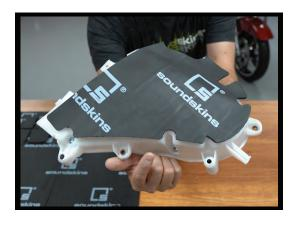
4. Then, move on to the left side pod. Piece 2 will go on the largest side of the pod. Line up the piece along the pod the same way you did on the right side, by aligning the screw holes that run along the side of the pod with the notches on the piece.
