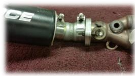
19. Rotate muffler and mid-pipe until the mounting bracket on the muffler lines up with the new foot peg adjuster plate mount.
