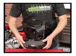
2. Piece 2 will go on the top side of the pod, you will find a flat section that pits the shape of the piece. You can tell which way the piece lays because of the square notches on the outer side of the pod.
