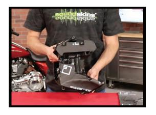
3. Piece 3 will go on the bottom of the side of the pod. To find where to start, line up the small protrusion from this piece along the area where it fits on the speaker pod. Mock the piece up before installing.
