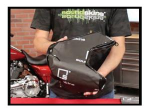
1. Start with piece 1. It will wrap around the fairing pod. The slit on this piece should come together when applied on the fairing speaker pods correctly. Mock up the piece to ensure proper placement before installing
