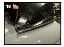
16. Once the Side Windshield Trim LED wires are plugged into the PT-HARN-14-JAE connectors tuck excess wires back into the hole where the PT-HARN-14-JAE wire was coming from. Shown in Figure 19.
