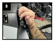
5. Remove vent cover by lifting up and out and set aside. Shown in **Figure 4.**
